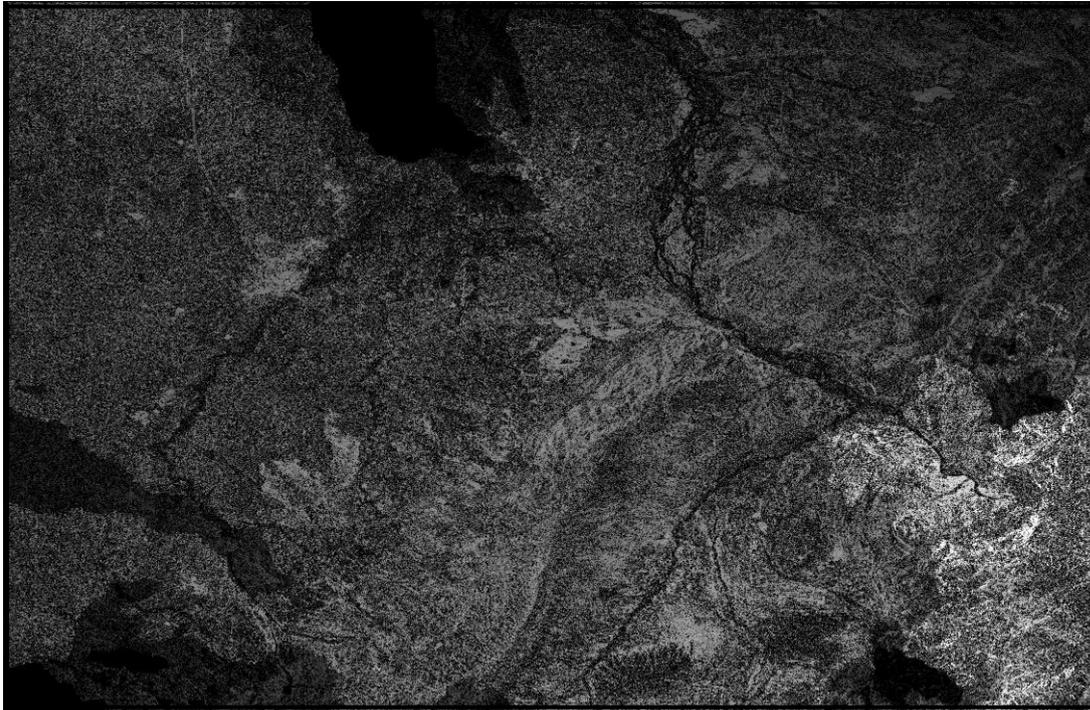
Figure 4.12: Phase unwrapped interferogram obtained from the first pair (Master image and Slave image 1)
