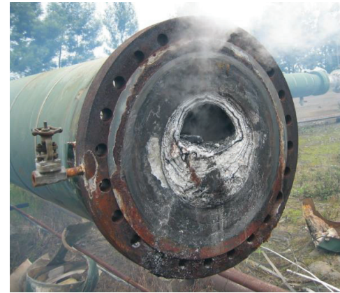
Figure 50 Typical problems found in the fields due to the impurity of geothermal fluid; silica scaling in pipes (left) and erosion on turbine blades (right)
