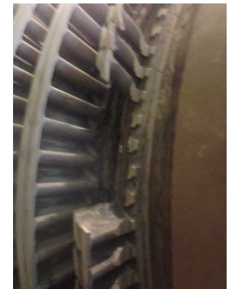
Figure 50 Typical problems found in the fields due to the impurity of geothermal fluid; silica scaling in pipes (left) and erosion on turbine blades (right)
