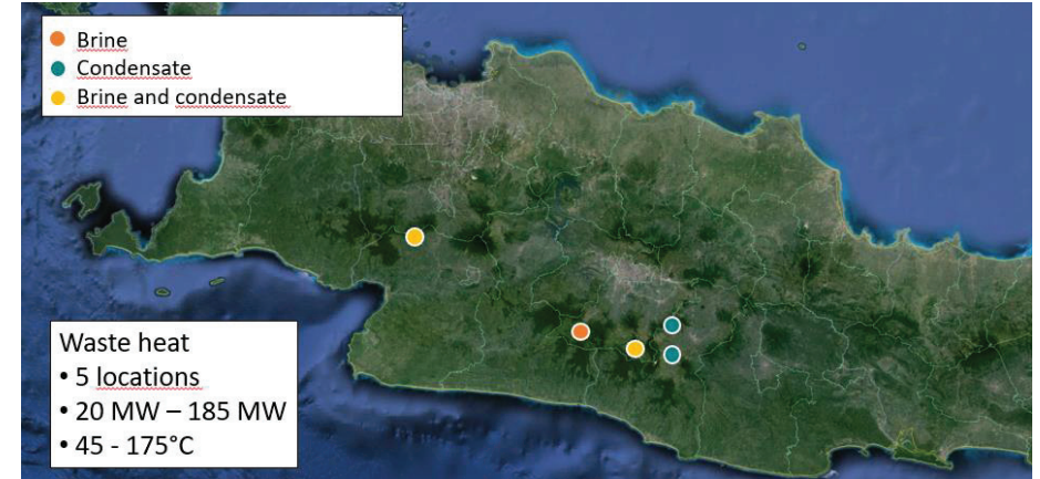
Figure 58 Locations of geothermal power plants with geothermal waste heat in West Java
