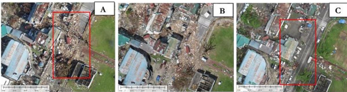
Figure 6.3. Uncertainty in assessing road damage as shown in different time series drone images. (A) image taken 6 days after the disaster showing the impassable road; (B) image taken 8 days after the disaster showing the cleaning up effort; (C) image taken 7 weeks after the disaster (Corephil Data Services Inc, 2013)
