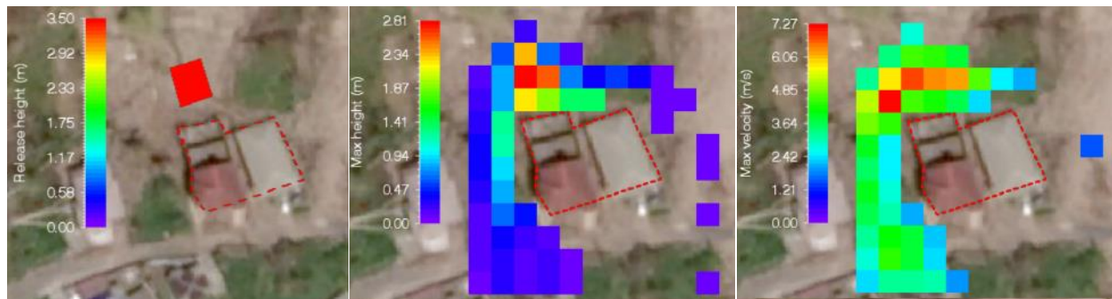
Figures 4.4– 4.6: (Left) The release depth was adjusted to 3.5 meters; (Center) simulation results in a max debris height of 2.81 meters and 2.0 – 2.5 meters of debris against the building; (Right) The velocity distribution shows a max flow velocity of 7.27 m/s and 4.85 m/s against the affected facade of Building 2.
