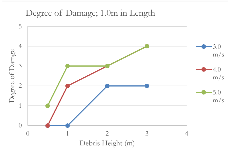
Figure 4.43a -4.43c: Adjusting the height of debris results in significant changes to the degree of damage at 1.0 meter; furthermore, increasing the velocity for debris heights over 1.0 meter significantly changes the degree of damage. (Top) The initial set up with a modelled element 11.0m in width and 1.0m in length and height for impact analysis; (Bottom) the simulated damage for a D2 classification at 4.0m/s. 1.0m video available at: https://www.youtube.com/channel/UCII_8TbvAsG2BZJENUtjcvg
