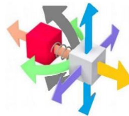
Figure 2.7: Visual representation of generic and spring constraints. The coloured arrows were edited from (Kostack, 2015), to show the six constraint types; Red & Yellow: compression and tensile; Blue & Purple: shear forces; Green & Grey: bending forces
