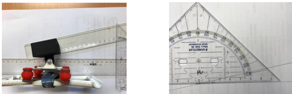
Figure 3.2 Measuring the tilt of the camera mounted in UAV using a protractor. The black part is where the camera was located.
