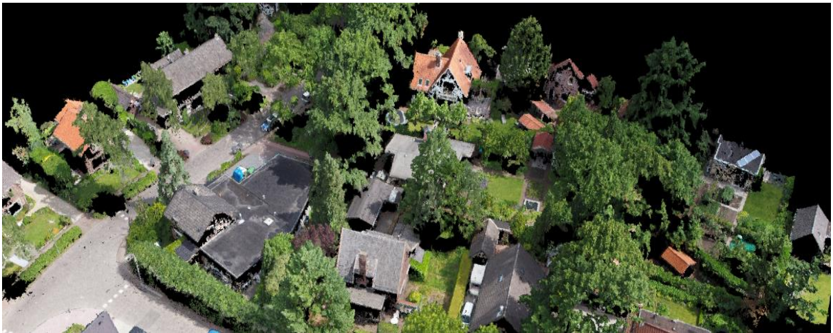
Figure 4-4 Showing trees covering the buildings roofs which needs to be filtered.
