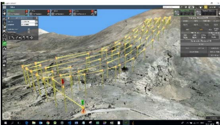
Figure 2.5: Interface of the UgCS software showing flight mission features. It enables terrain following mode flight mission planning
