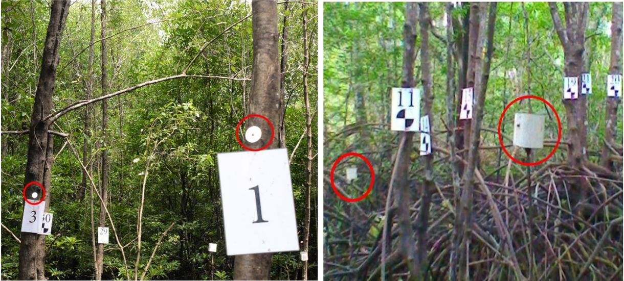
Figure 7. Both circular and cylindrical retroreflectors that used as a reference (the common point between the two-scanning position) to register all scanning position to a single data set. Circular (left) and cylindrical (right) retroreflectors used.
