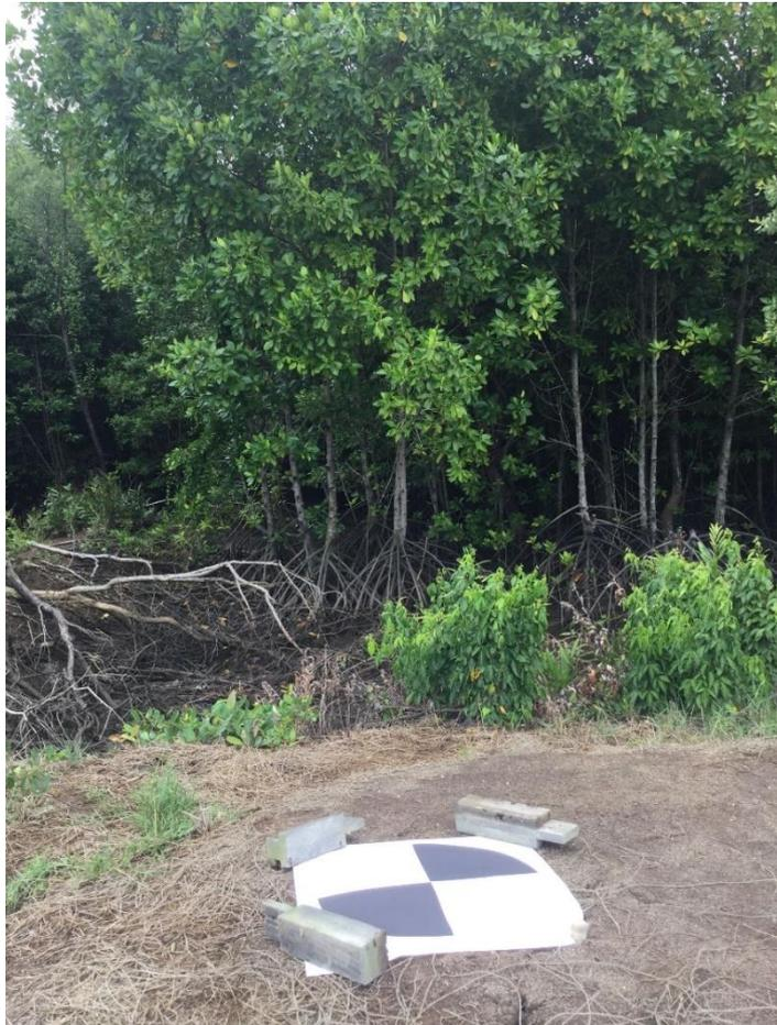
Figure 2.3 Ground Control Points (GCP) used in the study area before UAV flight.
