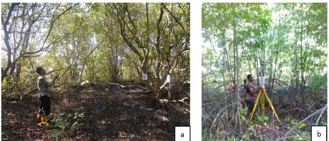
Figure 2.5 Measuring tree height using Leica Disto D510 laser ranger(a) and using TLS RIEGL VZ400 (b).
