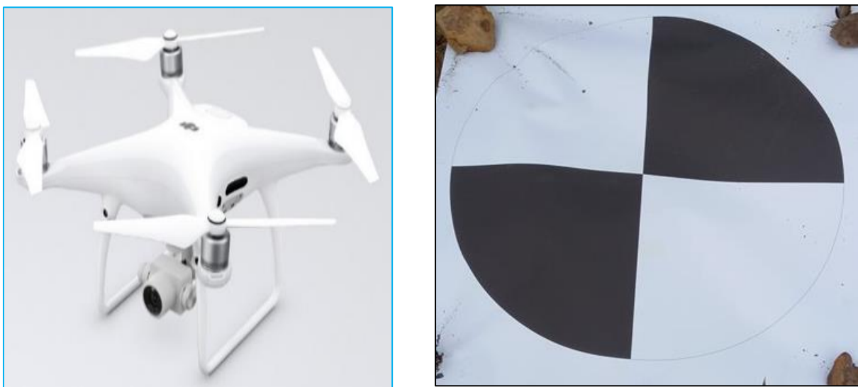
Figure 11: Phantom 4 DJI UAV-left, and GCP 60x60cm marker-right.
