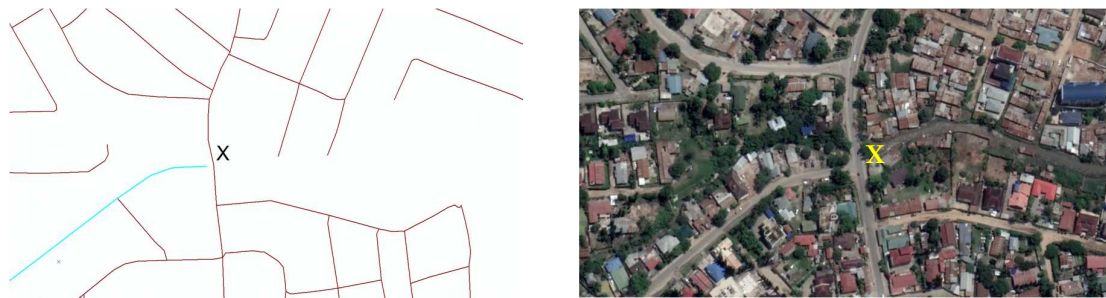
(i) (ii) Figure 3-9: Example of identified road junction at “X” (using ArcGIS software) not connected/undershoot (i), and its reality on the ground (ii)
