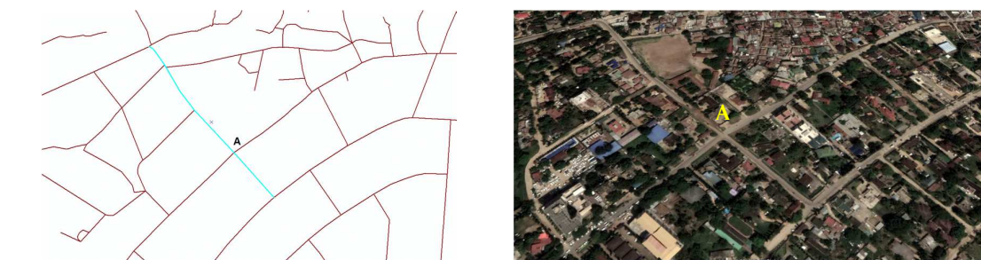
(i) (ii) Figure 3-10 Example of identified road junction at “A” (using ArcGIS software) not digitized as segment lines (i), and its reality on the ground (ii)
