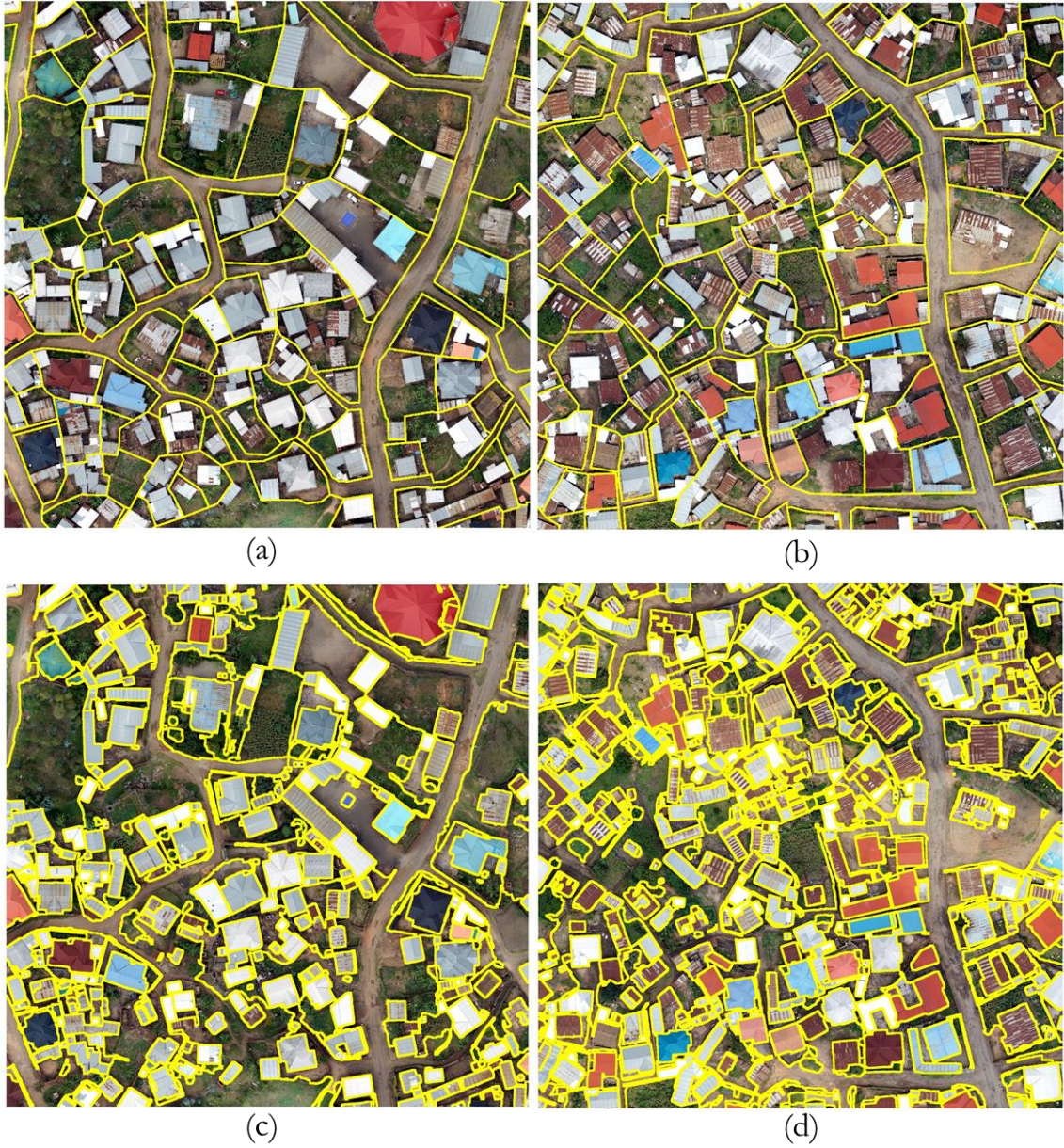
Figure 21: The detected boundaries of TS4 (c) and TS5 (d) in Muhoza using gPb-OWT-UCM. (a, b) are boundary references. The threshold of UCM is 0.3 in (c) and 0.1 in (d).
