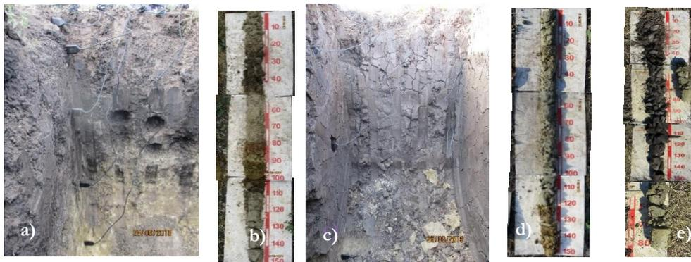
Figure 8 : Pits installed with soil moisture sensors in NPEW (a) and PEW (c) in plot 1; Bore logs of deeper profiles in NPEW (>120 to 250 cm) (b), PEW (>150 to 310 cm) (d) in plot 1 and PEW (e) in plot 2 (0-180 cm).
