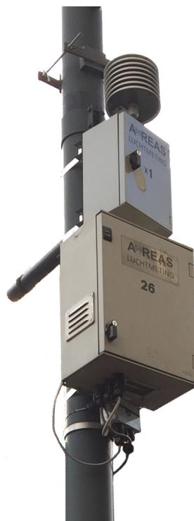
**Figure 2.3** Airbox attached to light pole.
