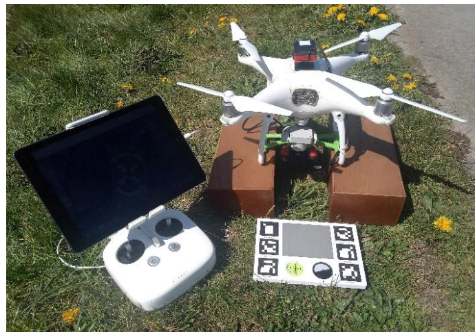
Figure 6. DJI Phantom 4 with Parrot Sequoia and sunshine sensor, the controller connected to a tablet and the calibration plate in the field
