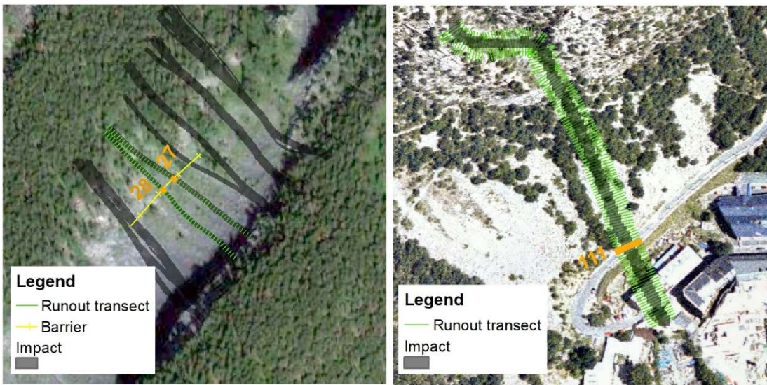
Figure 5-5 Delineation of the elements at risk and the selected transect within the runout axis
