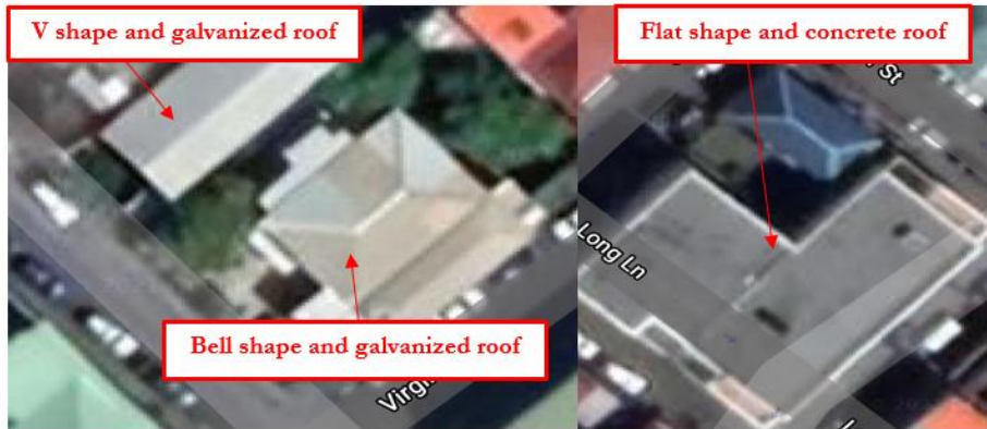
Figure 10: Type of roof shape included in the classification.
