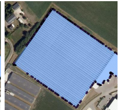
A predicted polygon with the tolerance of 9 pixels for polygonization Number of vertices = 395
