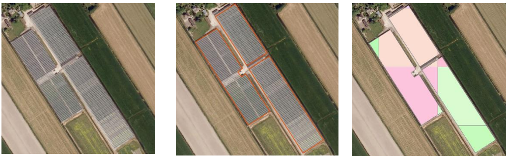
a) 0.1m ortho-image b) BRT reference data polygon c) Individual polygon per tiles
