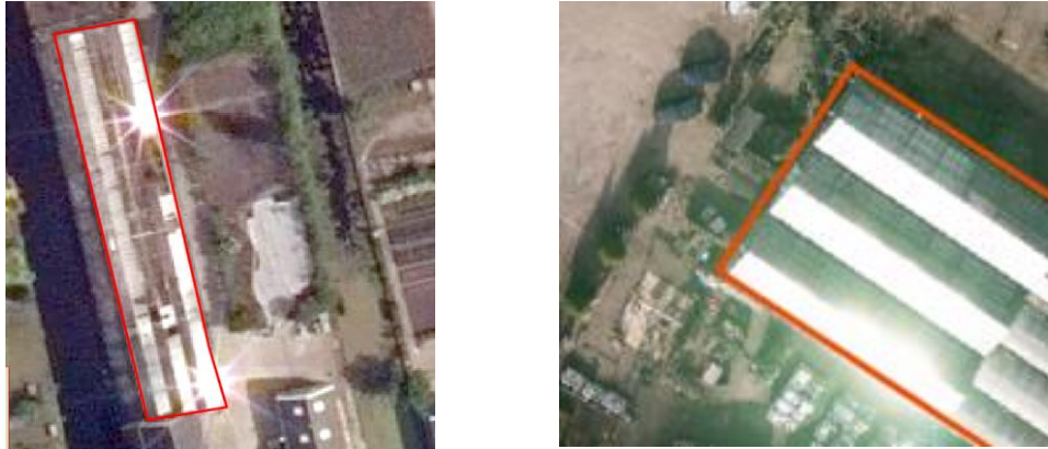
Figure 22: High-intensity reflection in a certain area of the greenhouse while taking an aerial image
