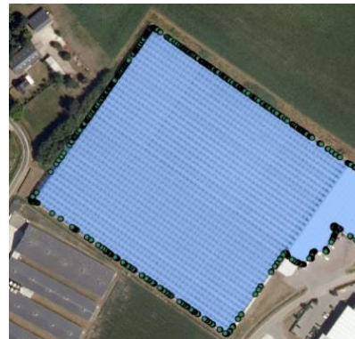
A predicted polygon with the tolerance of 1 pixel for polygonization Number of vertices = 674
