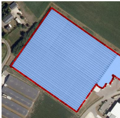
A predicted polygon with the tolerance of 0.125 pixels for polygonization Number of vertices = 1468
