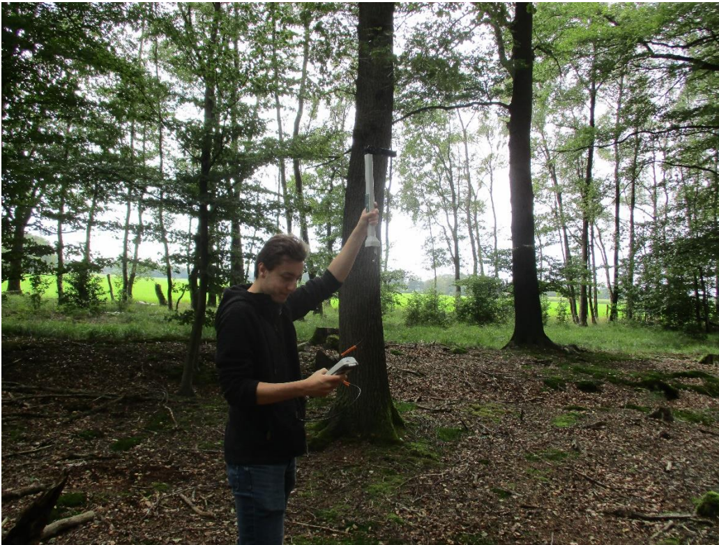
Figure 2: Below-canopy measurement of LAI using the LICOR 2200C.
