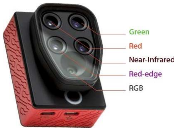
Figure 9: The Parrot Sequoia multispectral camera, with an indication of its five different sensors (©HORUS Dynamics).
