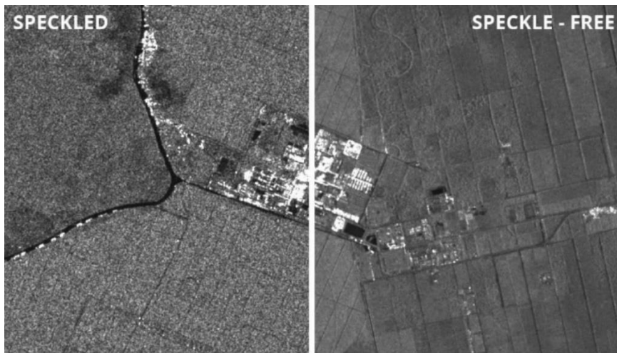
Figure 2-2: Speckled and speckle-free SAR images (Source: (“Speckle Filtering Pada Synthetic Aperture Radar - Bagas Setyadi,” n.d.))
