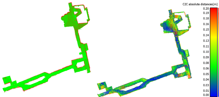
Figure 6.9. ITC-Backpack and TLS comparison. Left: Our point cloud (red) and TLS cloud (green) registered in the same coordinate system. Right: Our point cloud coloured based on the C2C distances to the TLS cloud
