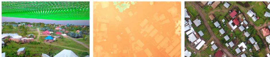
Figure A 5: Data products derived from UAV images. A: 3D point cloud; B: digital surface model; C: Orthophoto
