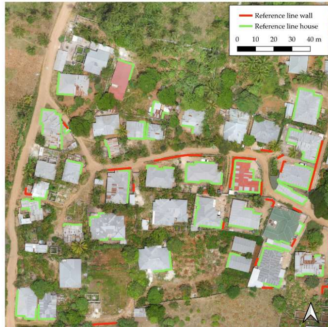
Figure 4.8: Selected reference lines representing rooftops (green) and walls (red) for the AOI in Kibonde
